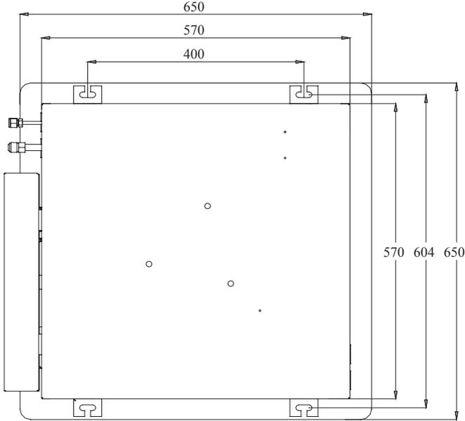
Fig.2 Install dimension of mode
